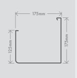
Fascia is used as a base to attach the roof guttering on to, or as a cover to hide the fixing space between the roof, eaves and wall. More than just functional, Fascia is designed to form a neat, attractive edge between the roofing and wall surface, as well as preventing birds and rodents from gaining entry to your roof cavity.
