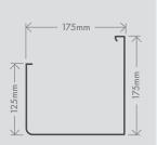
Fascia is used as a base to attach the roof guttering on to, or as a cover to hide the fixing space between the roof, eaves and wall. More than just functional, Fascia is designed to form a neat, attractive edge between the roofing and wall surface, as well as preventing birds and rodents from gaining entry to your roof cavity.
