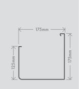
Fascia is used as a base to attach the roof guttering on to, or as a cover to hide the fixing space between the roof, eaves and wall. More than just functional, Fascia is designed to form a neat, attractive edge between the roofing and wall surface, as well as preventing birds and rodents from gaining entry to your roof cavity.
