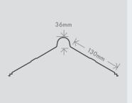
Our roll top ridge capping prevents rain or water from entering the house via the apex of the roof. It also prevents rainwater from penetrating the lower levels of a roof, which can damage the entire roof structure. Freeman Roofing ridge capping comes in a full range of colours and is made from genuine NZ made Colorsteel®
