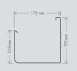
Fascia is used as a base to attach the roof guttering on to, or as a cover to hide the fixing space between the roof, eaves and wall. More than just functional, Fascia is designed to form a neat, attractive edge between the roofing and wall surface, as well as preventing birds and rodents from gaining entry to your roof cavity.
