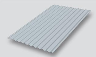
The minimum roof pitch for Corrugate is 8 degrees, and if end lapped, the pitch should be 10 degrees to ensure proper water drainage.
