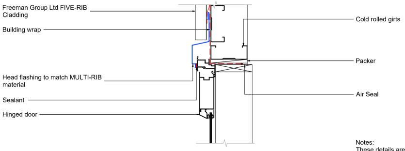
These details are required to be fixed to allow thermal movement.
