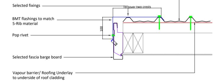
Notes: These details are required to be fixed to allow thermal movement .
